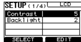
2. Rotate Knob 1 to select “Contrast,” and then rotate Knob 2 to adjust the legibility of the display.
