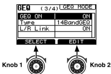
2. Rotate Knob 1 to select "GEQ ON," and then rotate Knob 2 to set to "ON."
