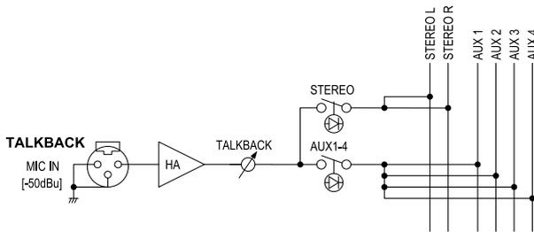
Use the talkback function to send instructions mainly from the operator to musicians and studio staff. This section adjusts the level of the microphone signal received from the TALKBACK MIC IN jack, and determines the bus to be output.
