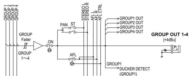
This section adjusts the level and controls the flow of the signals from the four GROUP buses. While the signal from each GROUP bus is always sent to the corresponding GROUP OUT jack, you are also free to use the ST and AFL switches to selectively send these groups to the STEREO and AFL buses.
