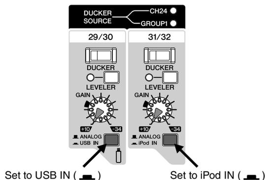
2. Turn on ( ) the **DUCKER** switch of the channel to which the device is connected in step 1, and then rotate the **GAIN** knob to adjust the input level of the channel.
