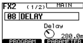
4. Turn on the ON switch of the input channel, and then rotate the FX2 knob to send the signal to FX2 RTN.
