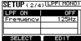
2. Rotate Knob 1 to select “LPF ON,” and then rotate Knob 2 to set it to “ON.”
