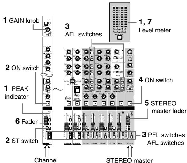
1. While producing sound on your instrument or microphone, adjust the channel GAIN knobs so that the corresponding peak indicators flash briefly at the highest peak levels.
