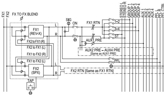
This section sets the effect returns (FX1 and FX2) on/off, and determines the level of the effect signal and to which bus the signal is sent.
