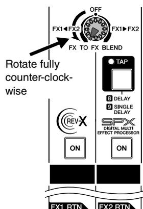
6. Turn on the ON switch of the FX1 RTN channel, and then raise the FX1 RTN fader to adjust the effect depth.
