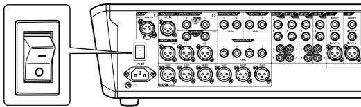
2. Connect the socket of the included power cord to the [AC IN] connector.
