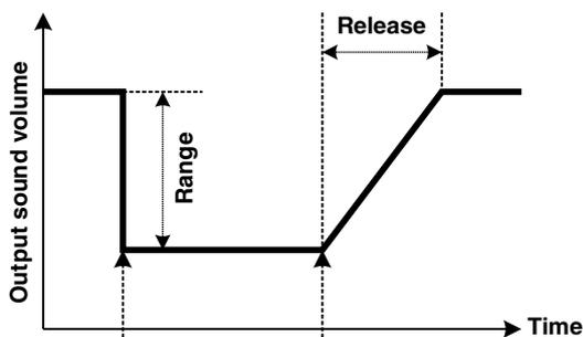
When the volume of the DUCKER SOURCE exceeds the threshold
