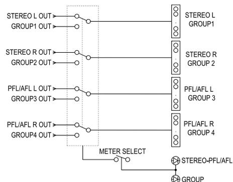
Use these meters to view various signal levels: the levels to the STEREO OUT L/R jacks, the PFL and AFL levels, and the levels to the GROUP OUT 1-4 jacks. The PFL or AFL signals indicated by these meters can be monitored through the MONITOR OUT jacks and the PHONES jack.
