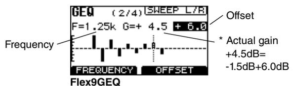
$$* \text{Actual gain} = \text{parameter (setting) value} + \text{offset}$$
