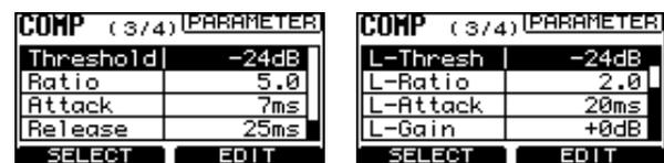
2. Rotate Knob 1 to select the desired parameter, and rotate Knob 2 to specify the parameter value.
