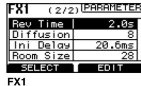
2. Rotate Knob 1 to select the desired parameter, and then rotate Knob 2 to set the value.
