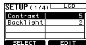
2. Rotate Knob 1 to select “Backlight,” and then rotate Knob 2 to adjust the brightness.
