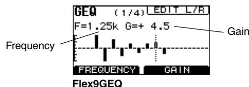
2. Rotate Knob 1 to move the cursor to the desired frequency.
