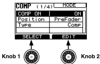
2. Rotate Knob 1 to select "COMP ON," and rotate Knob 2 to set to "ON."
