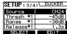
5. Confirm that “Source” is selected, and then rotate Knob 2 to set the input source to “CH24 {CH16}” or “GROUP1.”
