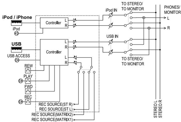
This section determines the destination of the signal output from the connected USB device or iPod/iPhone, and adjusts the signal level.
