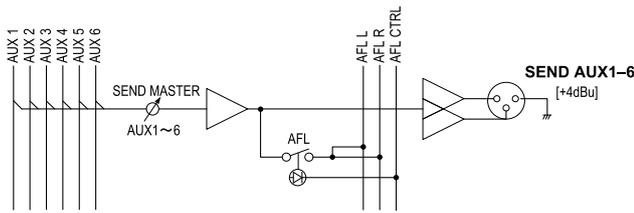
This section adjusts the levels and controls the output of signals from the six AUX buses. Each of these signals outputs to the corresponding SEND (AUX1-AUX6) jack respectively.
