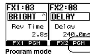
2. Rotate or press Knob 1 for FX1, and Knob 2 for FX2.
