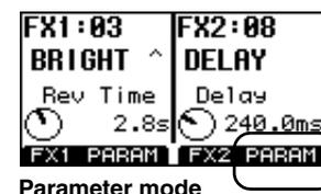
2. Rotate Knob 1 (for FX1) or Knob 2 (for FX2) to adjust the parameter.
