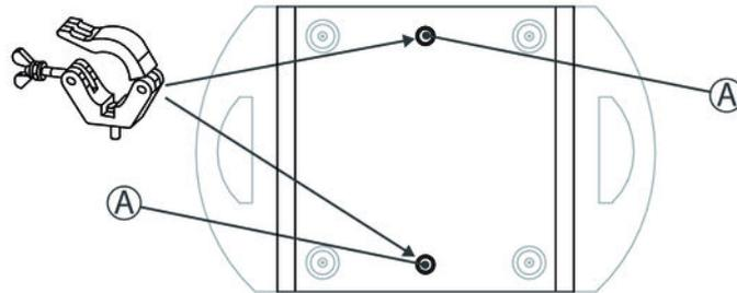
A Quick lock openings for Omega brackets
